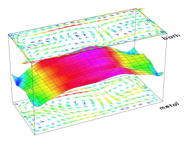
Figure 5: Flow field in the metal and bath and metal/bath interface contour
