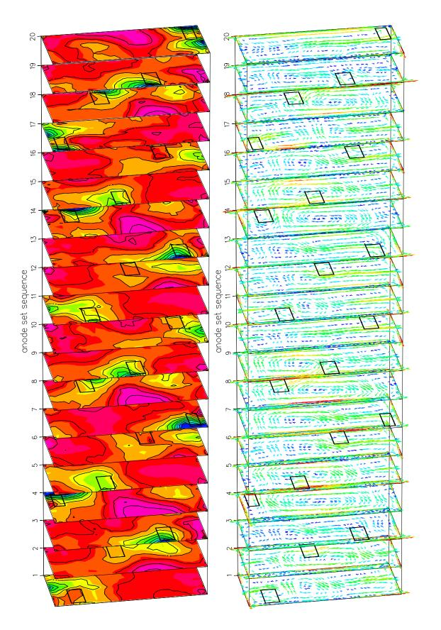
Figure 6: Anode-cathode distance distribution and fluid flow in the metal during a complete anode set cycle (rectangles indicate position of the new anode)
