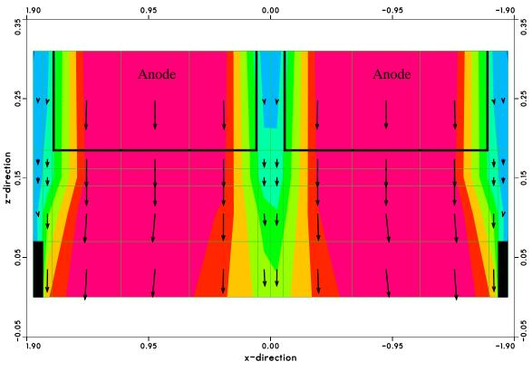
Figure 4: Electrical potential and electrical current density - sectional view
