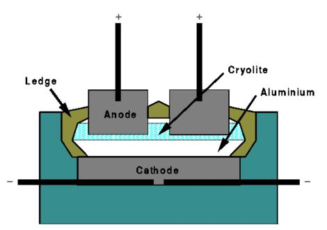
Figure 1: Cross-section of a alumina reduction cell - schematic drawing
