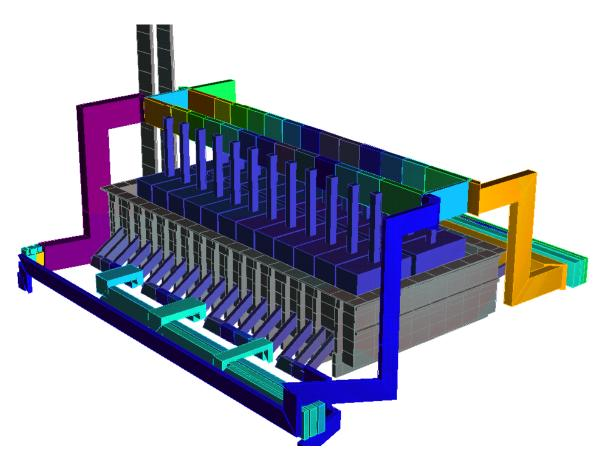
Figure 2: Simulation model of a reduction cell
