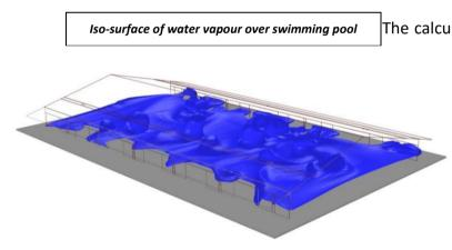
The calculation mesh had a total of 7 million grid points, with the majority in the region containing the natatorium. This provided sufficient refinement to resolve the geometry adequately and capture flow detail within the natatorium. The modified K- $\epsilon$ model of Chen and Kim was used to represent turbulence.
