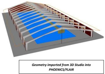
A 3D-Studio engineering CAD file was imported into PHOENICS/FLAIR via the inbuilt AC3D utility, and the major features of the natatorium were included in the model.
