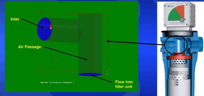
An approximation of the current Walker Filtration inlet design in the PHOENICS VR viewer. The inlet has a diameter of 20mm and is pressurised to 3Bar. The working fluid at the inlet is air at 20<sup>o</sup>C.
