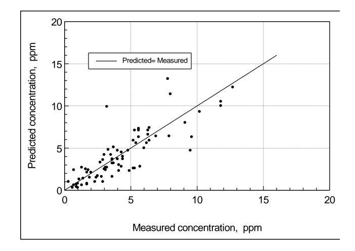
Comparison between predicted and measured CO for windward face of downwind building, Hope Street, Glasgow
