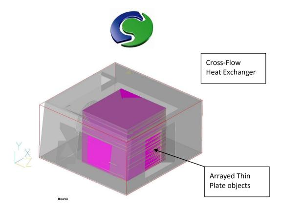
RMS engineers were primarily interested in using the CFD model to calculate and predict the thermal performance and effectiveness of the VMS heat exchanger under different boundary conditions (such as different internal or external inlet temperature, different air flow rate for exhaust fan etc) and how would they affect the results.
