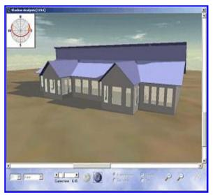
The room geometry information, including the surface temperatures and convection coefficients, together with room objects like diffusers and heat sources, is created parametrically in Hevacomp's new Simulation module. The complete input file is then passed to the CFD solver provided by CHAM. A key issue is the accurate modelling of diffusers and grilles. CHAM in co-operation with Hevacomp has implemented diffuser objects based on ASHRAE research.
