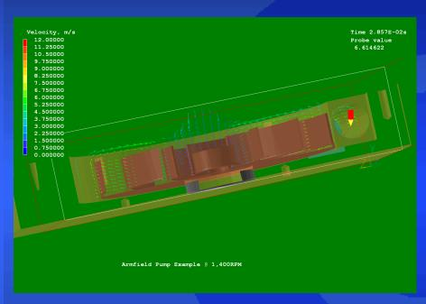
Velocity vectors within the pump, showing use of the 'near-plane' function to view inside the impeller cross section.
