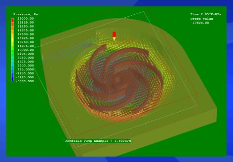
Sectional pressure profile and vectors through and around the impeller.
