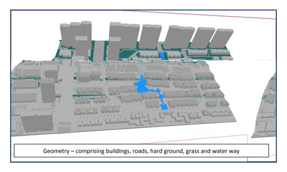
The idealised geometry shown above contains many of the components of interest to the "Heatisle" engineer; viz, concrete and glass high rise buildings, tarmac roadways, hard terrain and vegetation, and a water course. Each component responds differently to solar radiation.
