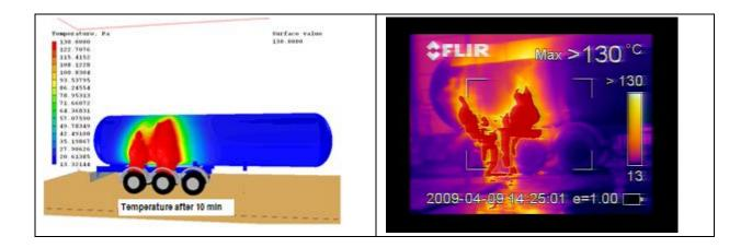
Comparison at 5 min and 10 min : computation and experiment (infra red camera)
