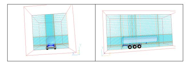
The comparison was made on the first half-hour of the experiment. In the computation, the fire was represented by a volume source term. The heat release rate of the tire was deduced from measurements of heat fluxes. The following figure presents a comparison of the wall temperature above the central tire. The computation result is in good accordance with the experimental results.
