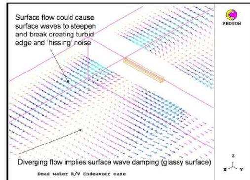
Figure 5. Close up view of near field surface flow vectors (colour coded) showing circulations of opposite sign in the bow and stern internal waves.
