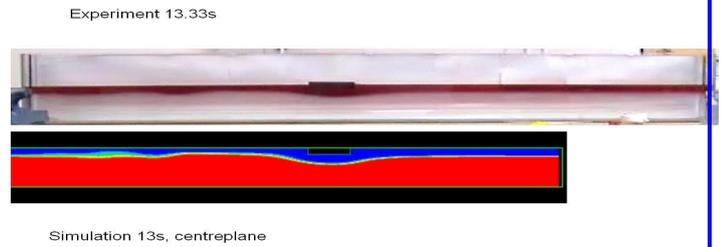
Figure 3. Comparison of experiment (top) at 13.33s and the PHOENICS simulation at 13s for a rectangular boat shape. In the experiment the upper less dense layer is dyed red and overlays denser fluid (no dye). In the PHOENICS simulation the less dense fluid is coloured blue and the dense fluid coloured red. The boat is travelling from left to right.
