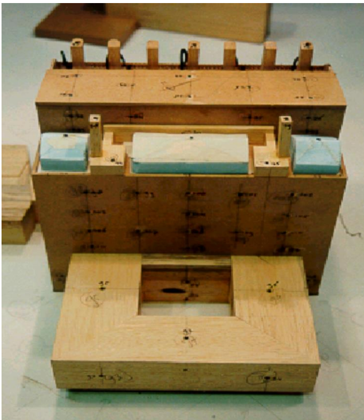
Figure 9: wind tunnel model of Biosciences Centre Liverpool
