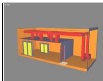
A plant room; some work is needed to merge the pipework into a single object and correct the pipes shown here
