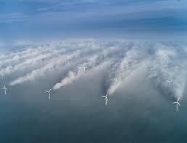
Figure 2. Horns Rev 1 is an 80 turbine wind farm off the western coast of Denmark, commissioned in 2002, and delivering 160MW. The above photograph shows the turbulence field downstream of the wind turbines. Unique meteorological conditions on 12 February 2008 at 1300 hours resulted in the wind turbines creating condensation (i.e. clouds) of the very humid air, thus making it possible to see the turbulence pattern behind the wind turbines.
