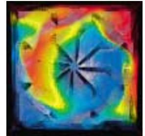
Above & Front Cover: Head on view of mixing of hot and cold air through end and side vents behind an air blending vane. Below: Streamlines - side view. Pictures courtesy of Air Blender Inc, Colorado, USA.
