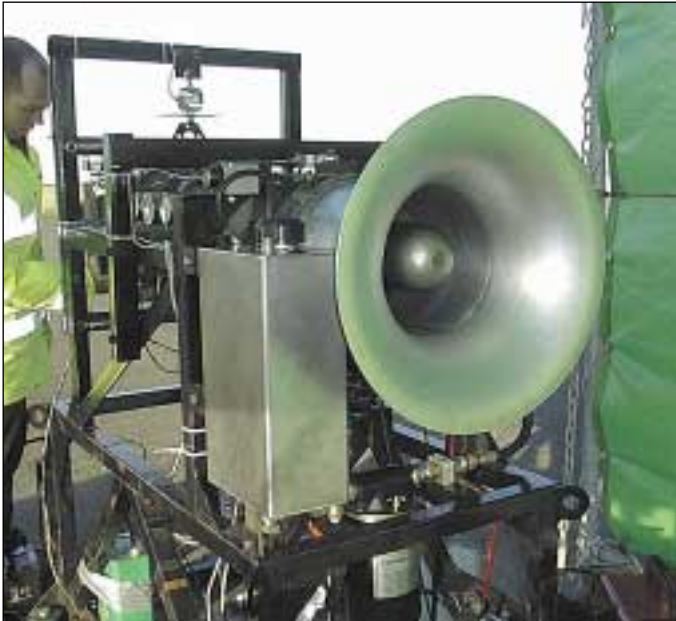
Intake of Gnome Gas Turbine
