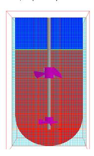
PHOENICS software was used with MOFOR to simulate the rotation of the impeller. The study was conducted in four steps:
