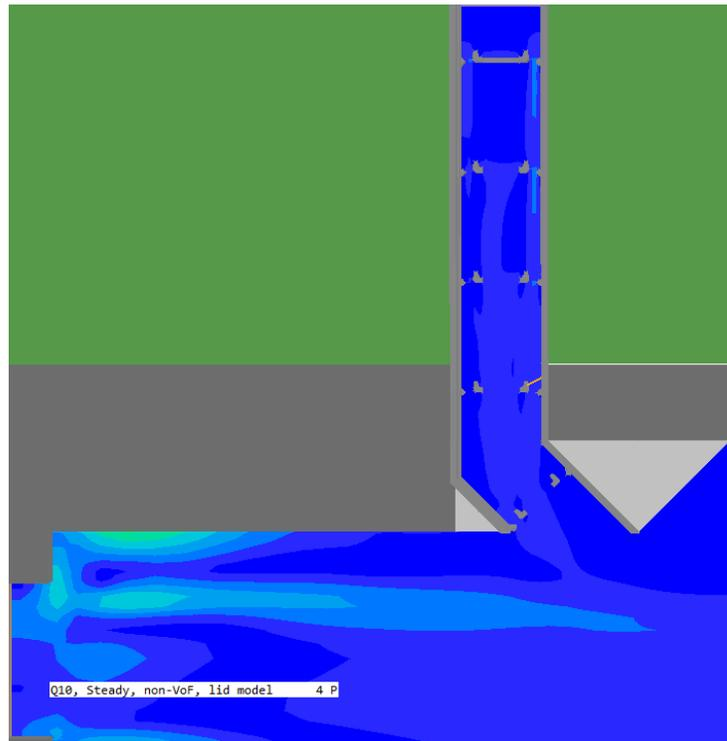
Case 3 looks at the region downstream of the sluice gates and around the fish pass' outflow. The model includes the last 5 (out of 20) sluice gates of the fish pass. It is a steady-state simulation, run for several water heights with different configurations for the number and the location of open sluice gates. It was investigated to establish if the velocities at the base of the fish pass were conducive to attract fish.
