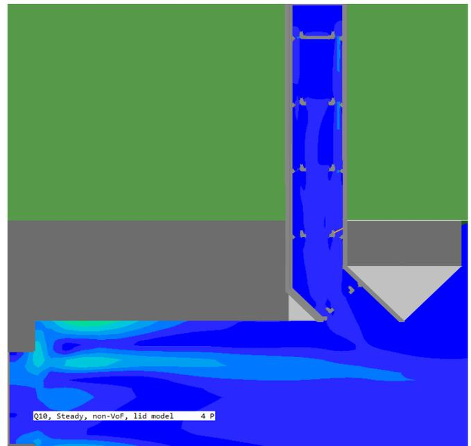
**Case 3: post-weir river velocity – fish pass exit – plan view**
