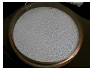
Figure 13: Photo of Rayleigh-Bénard experimental set up with a free upper surface (From John Matsson, thesis).
